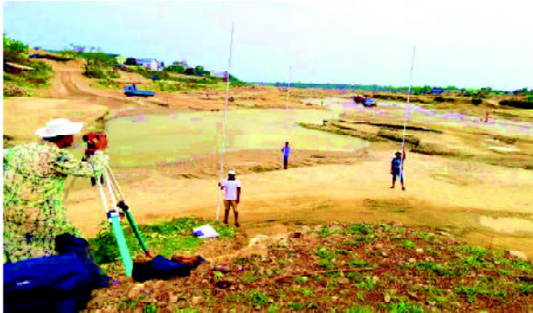
Photo 1: RL survey on Rakti River at the confluence of Rakti and Balason River by auto level on 15/04/2019
