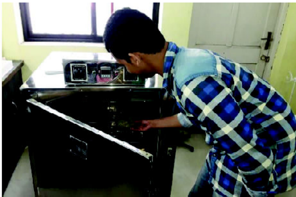
Photo 3: Sediments are dried by hot air oven at 100° centigrade (28/05/2019).
