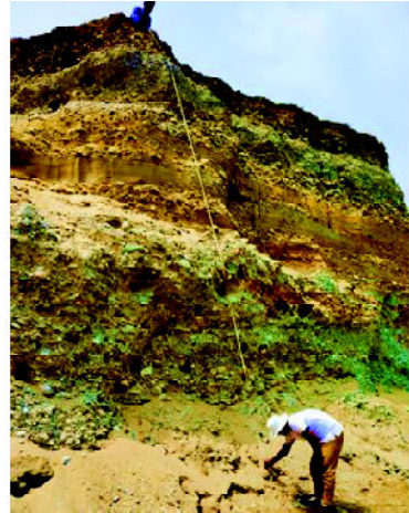
Photo 2: Collection of the bank sediment from different layer and measuring the bank height by measuring tape.
