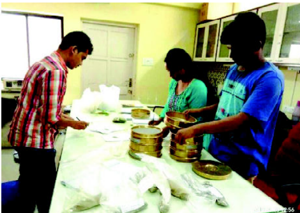
Photo 5: Labeling and packing of sediment samples, classified into several phi classes by using digital sieve shaker (28.05.2019)
