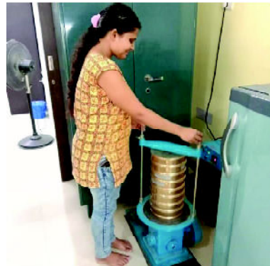
Photo 4: Sediment samples are classified into several phi classes by using digital sieve shaker (28/05/2019).
