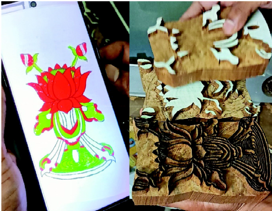
Fig. 4. Multi-coloured blocks are prepared separately as per the number of colours, (here it is black outline, red and green) as done by the sons Mr. Pragnesh Prajapati and his brother Avdesh Prajapati.
