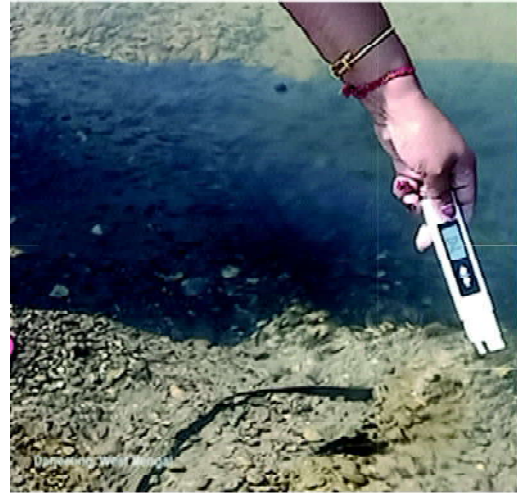
Photo 19: Using field kit to measure the chemical parameters of the water sample collected from Chamta channel
